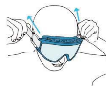
Pic.2 - Set the length of the elastic band by gently pulling back the ends
